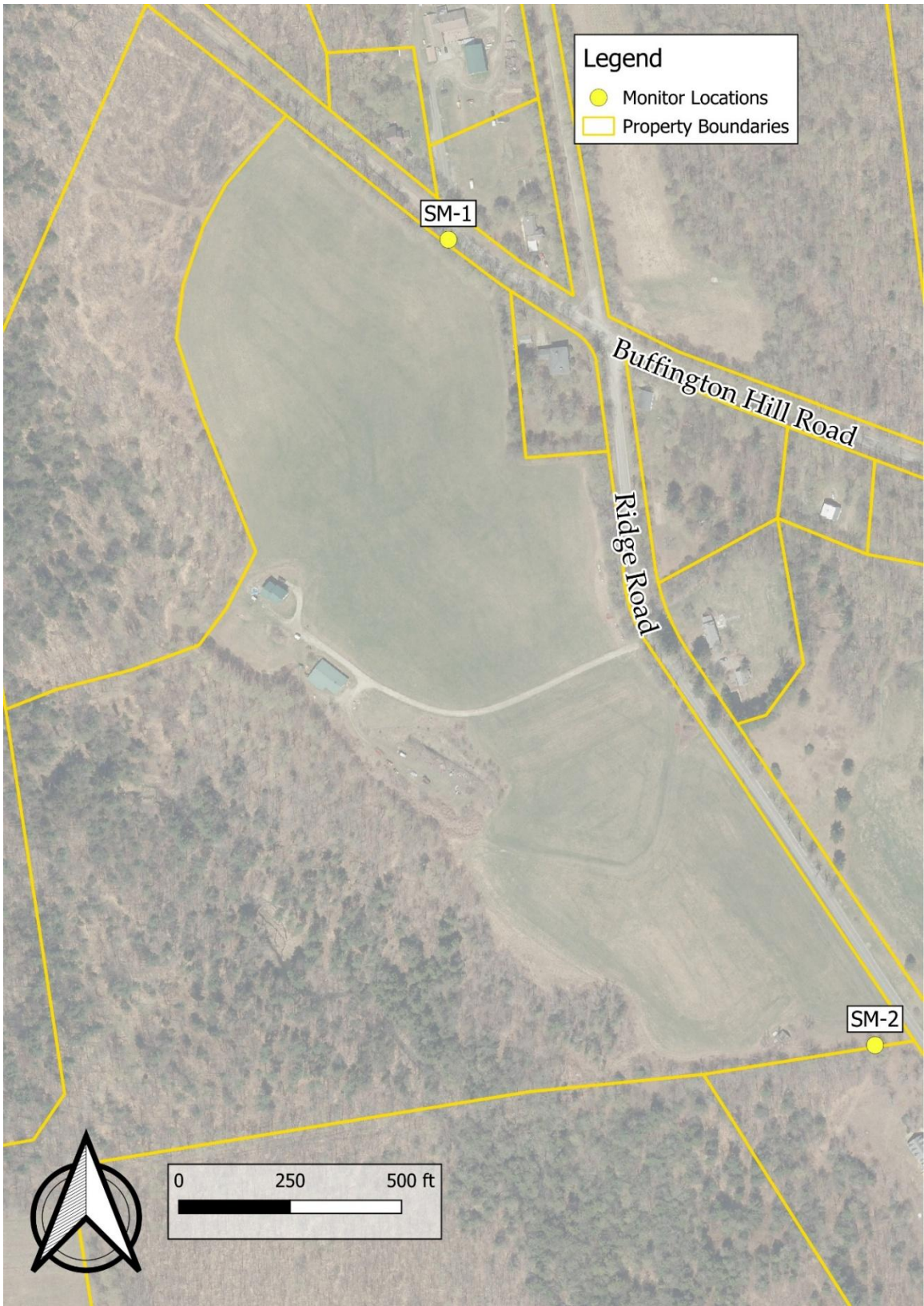
Aerial Photograph of Project Area Indicating Location of Sound Monitors
