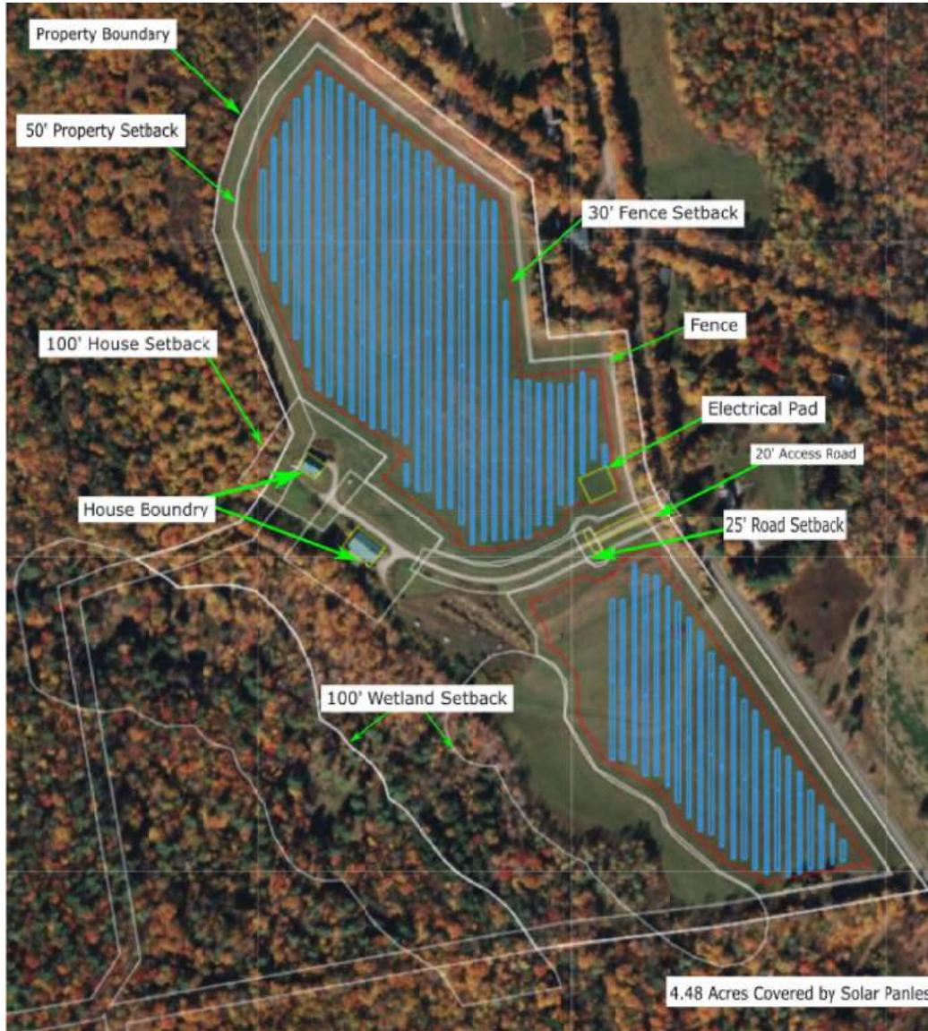
1 PROPOSED GROUND MOUNT PV ARRAY 3.84 MWDC: 1.99 MWAC
